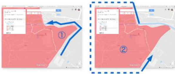
Figure 10. To combine two regions, sequence of control points not included in the border are merged into one sequence of points.
